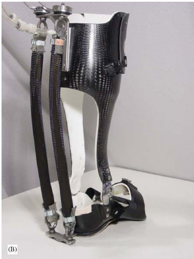
Fig. 1. Powered ankle-foot orthosis. Each ankle-foot orthosis consists of a custom fit carbon fiber shank section and a polypropylene foot section. Load sensors in series with the artificial muscles monitored artificial muscle tension. (A) An orthosis fit with a single artificial pneumatic muscle to provide plantar flexion assistance. (B) The same orthosis fit with two artificial pneumatic muscles in parallel to provide plantar flexion assistance. All artificial muscles pictured are in a relaxed state.
